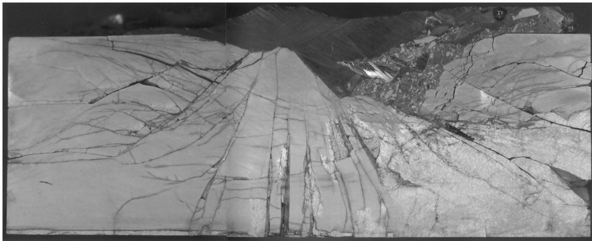
Fig. 25. Recovered \text{TiB}_2 disk from shot 7-1803 showing more damage compared to that in experiment 7-1800. Mixing of WHA material with \text{TiB}_2 fragments is less pronounced than in the case of the \text{Al}_2\text{O}_3 target.
