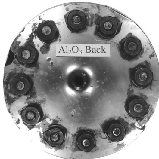
Fig. 9. Photograph of the bottom surface of recovered steel back plate from experiment 7-1797 ( \text{Al}_2\text{O}_3 ceramic).
